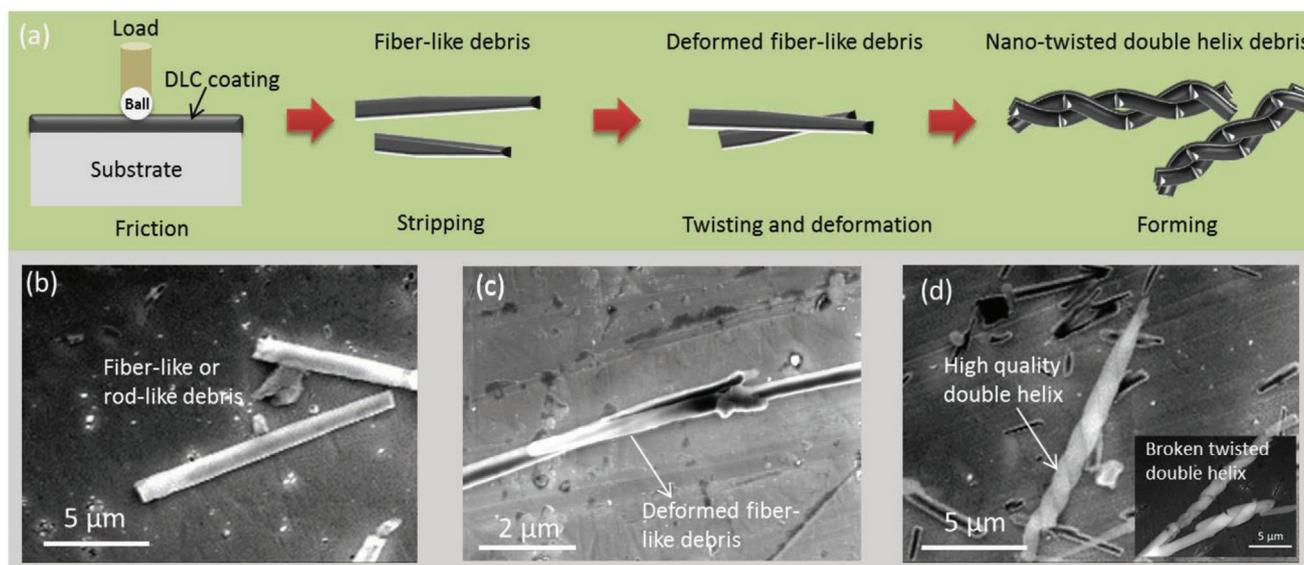
**Figure 8.** Schematic diagram of the formation mechanism of a) nano-twisted double helix wear debris and b–d) typical SEM images of the wear debris of the Si-16 coating.
