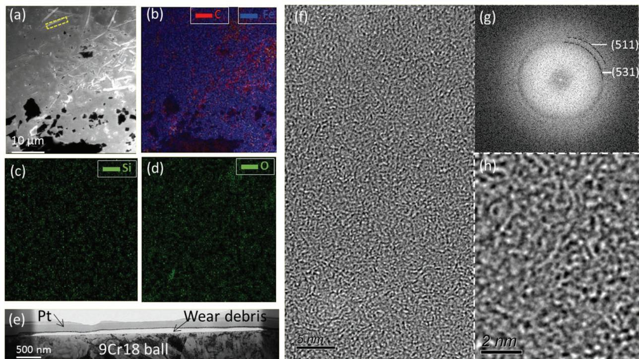
**Figure 7.** FESEM image a) and EDS mapping result b–d) of the wear debris of the Si-16 sample. e) The corresponding TEM debris sample made by FIB lift-out method. f) The corresponding HRTEM images of the wear debris. g) The corresponding FFT image. h) The magnified view of the HRTEM image of the wear debris.
