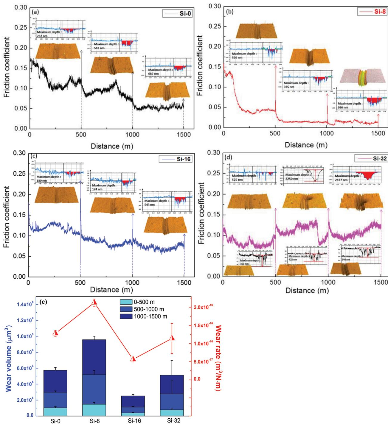
**Figure 4.** a–d) Friction coefficient, wear morphology and e) wear rate of the as-deposited coatings.
