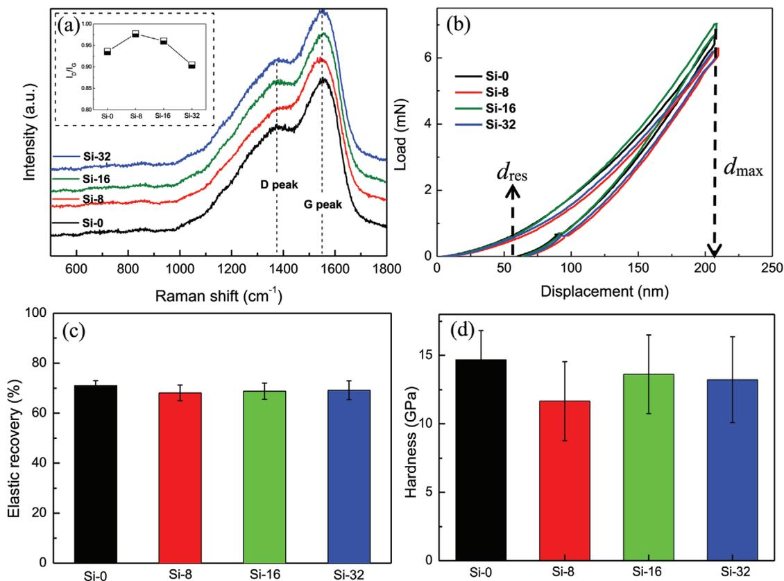
Figure 2. a) Raman spectroscopy and b) load-displacement curves of the prepared coatings, c) the results of elastic recovery and d) hardness of the coatings during the nanoindentation test.
