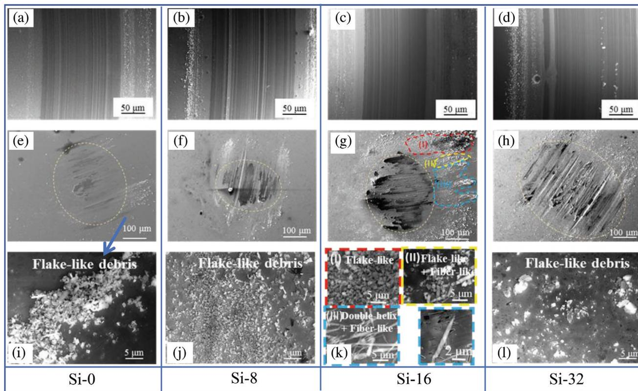
**Figure 5.** a–d) SEM images of the wear tracks on the coating surface and e–h) the friction pair. i–l) The wear debris on the corresponding friction pair.
