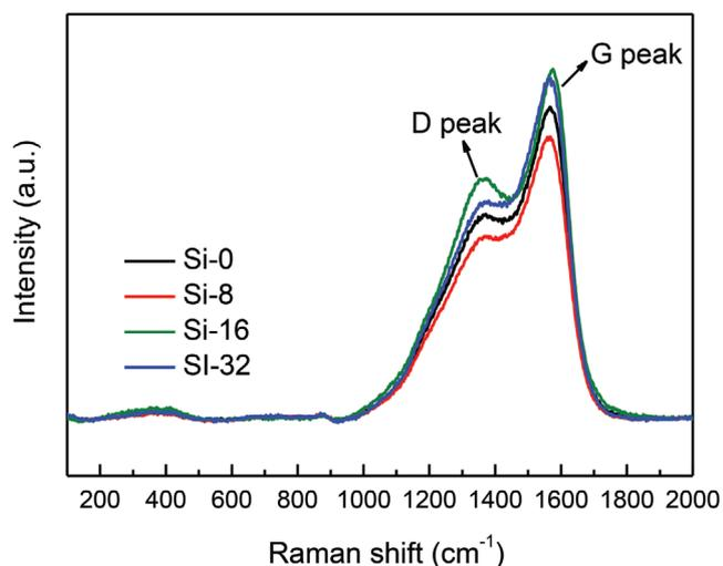
**Figure 6.** Raman spectroscopy of wear tracks of the deposited coatings.
