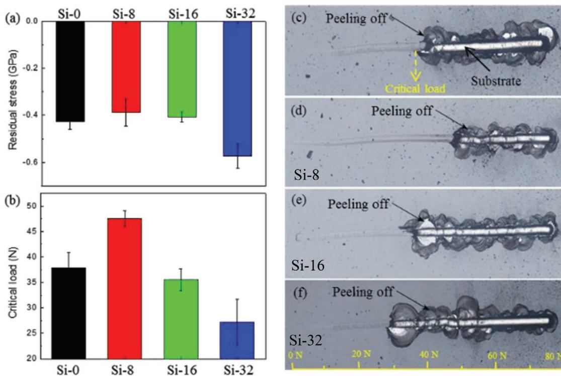
Figure 3. a) Residual stress and b) critical load of the as-deposited coatings, c-f) the corresponding scratch morphology of the coatings.
