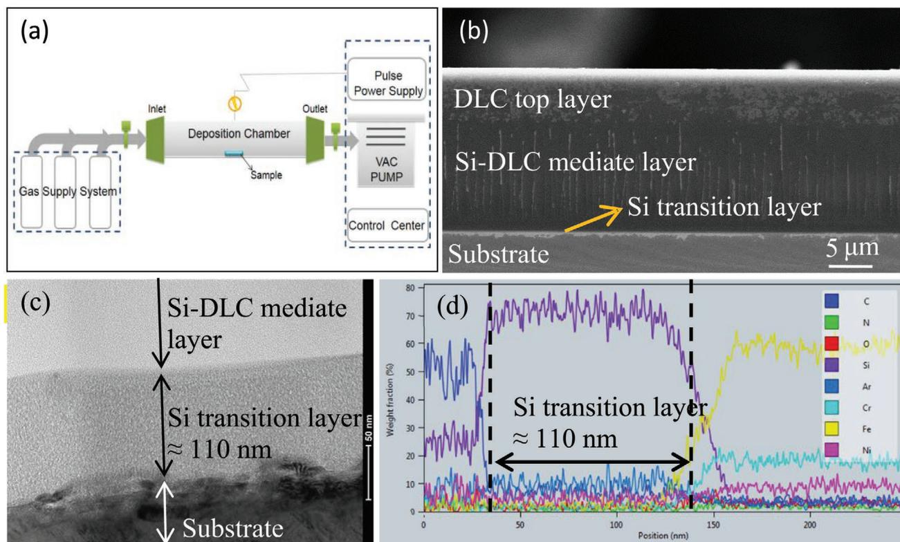
**Figure 1.** a) Schematic diagram of a hollow cathode plasma immersion coating system. b) The SEM cross-section image. c) TEM cross-section of the Si-8 sample and d) the corresponding EDS line scan result.
